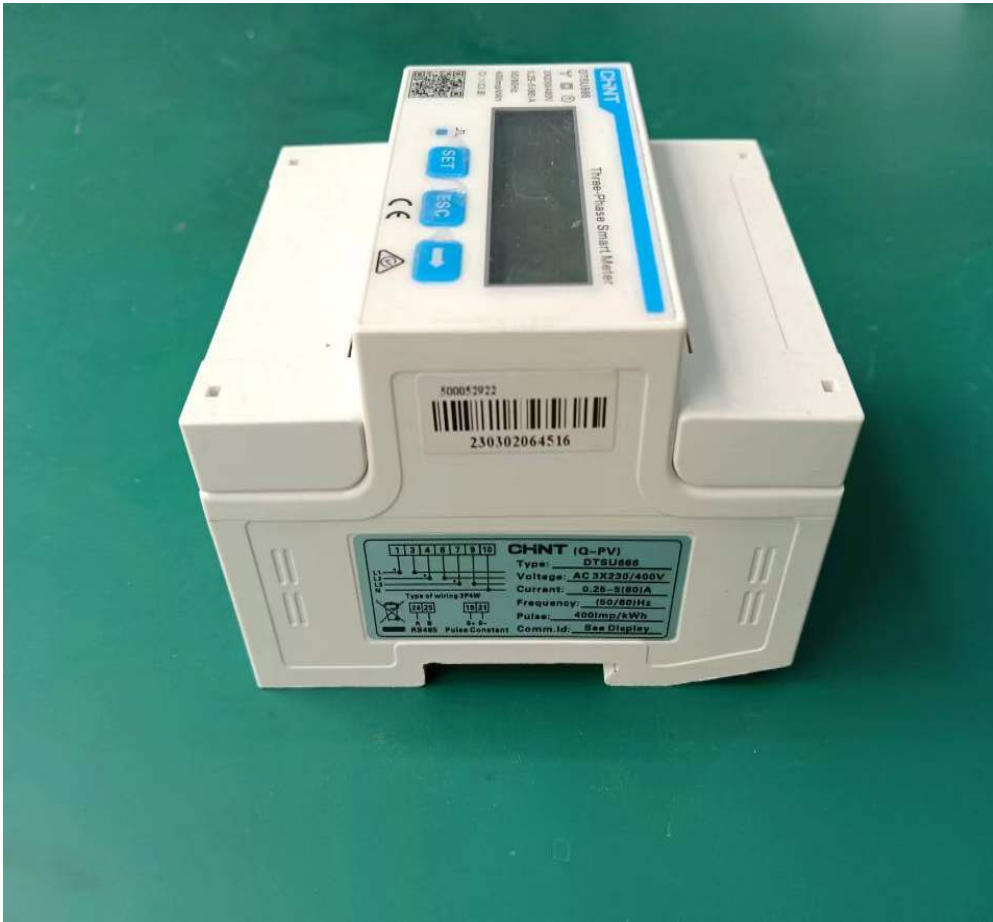
The energy meter (CLS) view
