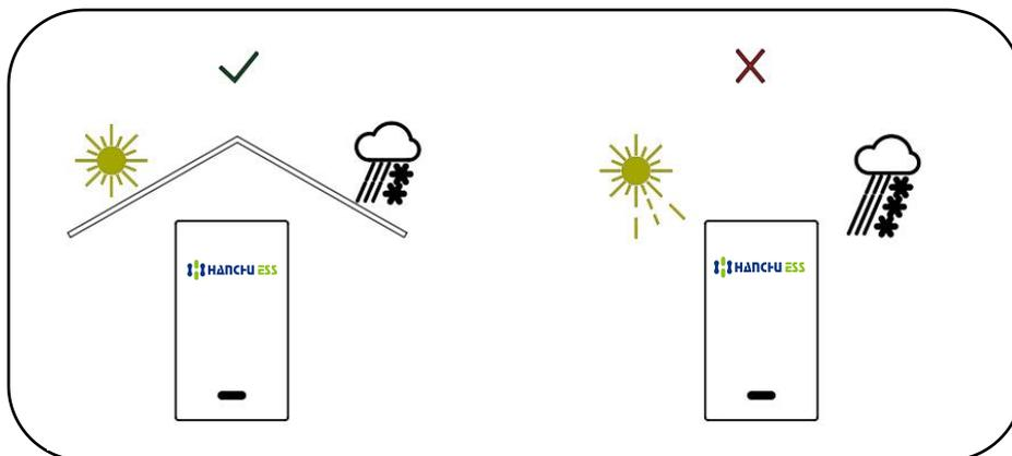
Figure 4 Installation Environment
