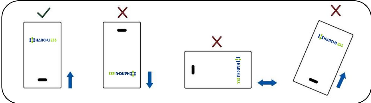
Figure 5 Installation Angle
