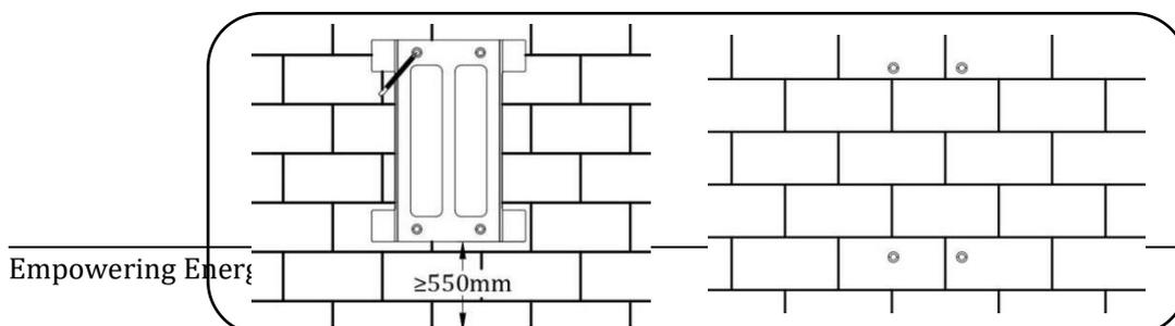
**Figure 9 Sample of Step 1 For Wall Installation**
