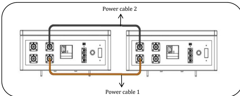
Figure 15 Sample of Power Connections Between Batteries
