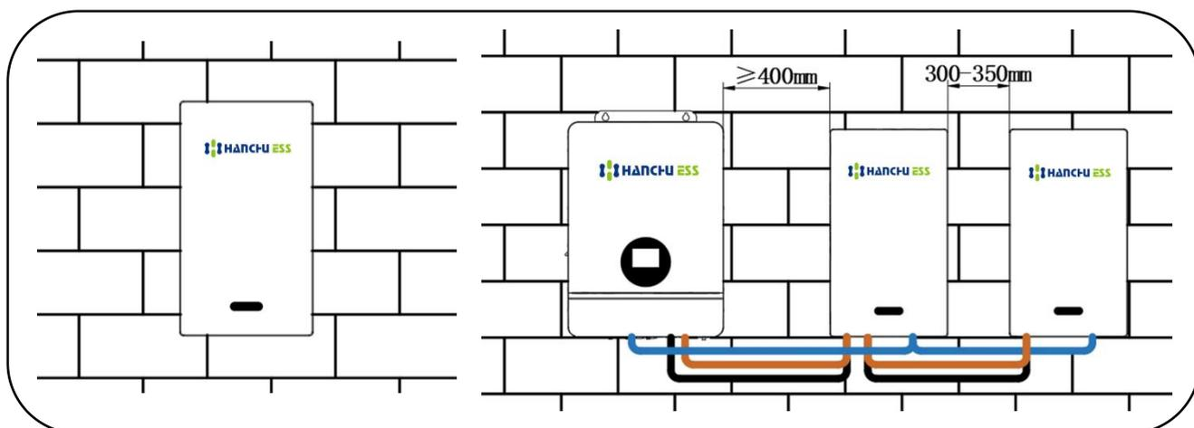
**Figure 11 Sample of Step 3 For Wall Installation**
