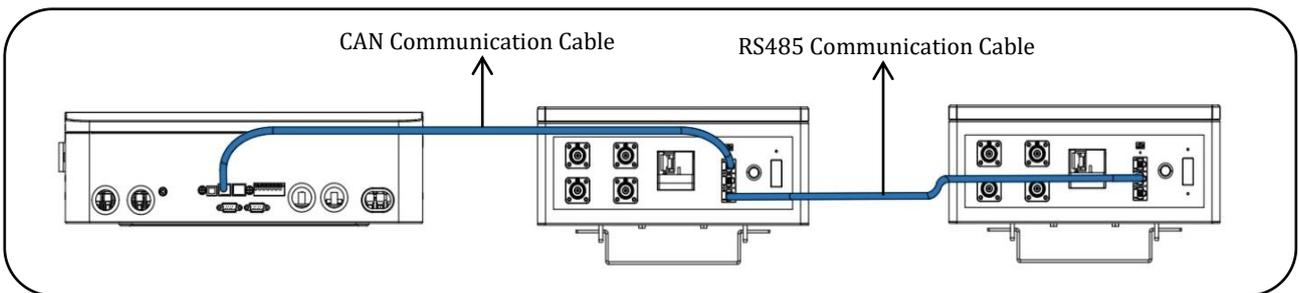
**Figure 17 Sample of Connection for the Communication Cable**
