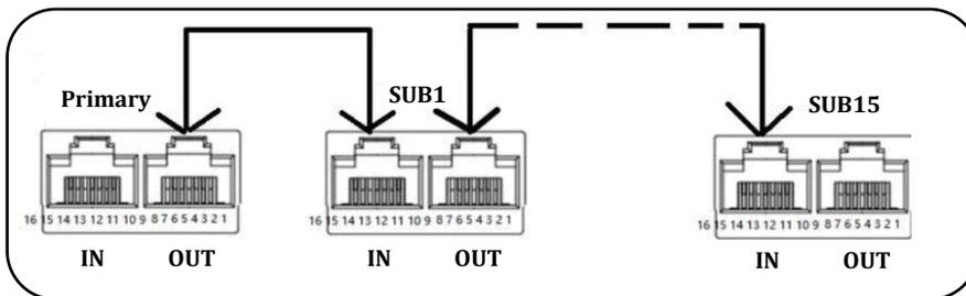
**Figure 18 Sample of Communication Parallel**
