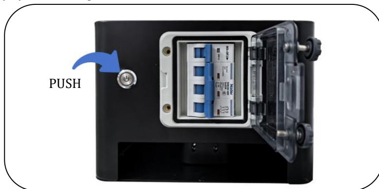
Figure 32 The Power Switch Of Battery Systems
